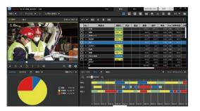
Analyze multiple targets on one screen. Its applications include analyses of cooperative work up to five people and of multi machine handling, as well as therblig analyses.
