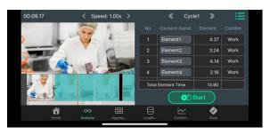
The video captured can be used directly to perform a time study and work analysis, and to improve productivity by eliminating waste, inconsistency and worker overburden while on-site.
