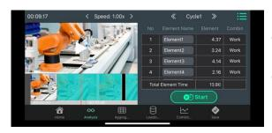
Slow-motion playback can identify time wasted in 0.1-second increments, and appropriate tuning can lead to increased productivity.
