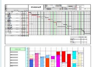
Utilize the analyzed data for your high accuracy work composition. **Output simulated results as** Standardized Work **Combination Chart.**
